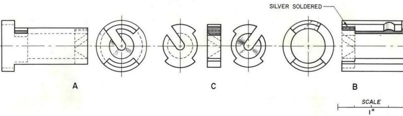
Fig. 3 Diagram of tensile yoke.
